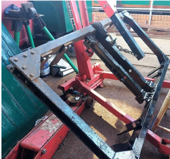
Replacement Frame receiving coat of smooth Hammerite (Photos Alan Titheridge)
