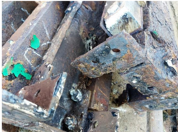
Original frame removed and ready for scrap, showing deterioration (Photos Alan Titheridge)
